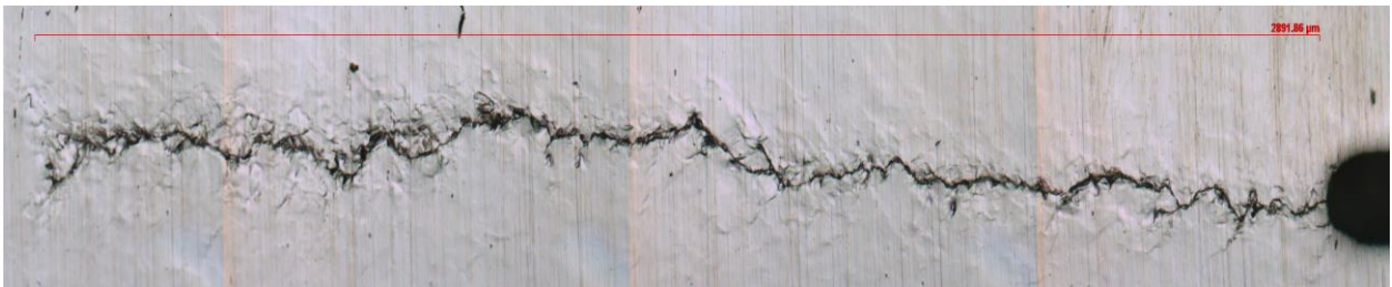
Figure A.9. Micrograph of the fatigue crack at 80000 cycles of 2.89 mm.
