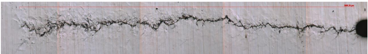
Figure A.10. Micrograph of the fatigue crack at 90000 cycles of 3.69 mm.
