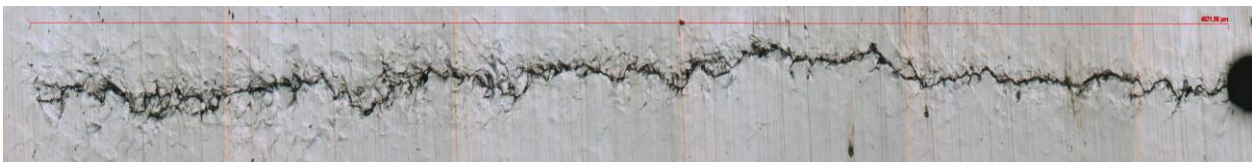
Figure A.11. Micrograph of the fatigue crack at 100000 cycles of 4.82 mm.
