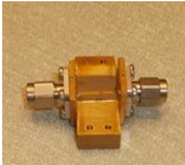
Figure 4.3 Photography of a microstrip gapline switch [4.1] for top illumination
