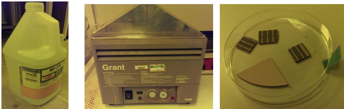
Figure 3.13 MF319 Developer (Left), Bath Heater (Middle) and Etched Wafers (Right)
