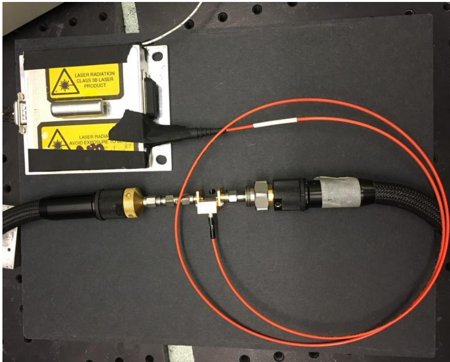
Figure 3.6 Measurement setup with optical illumination provided by fibre-coupled laser
