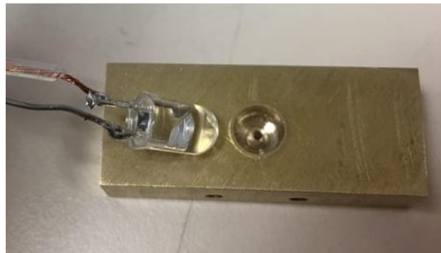
Figure 6.13 IRED connected by DC wires and brass block with a 6mm diameter hole for mounting
