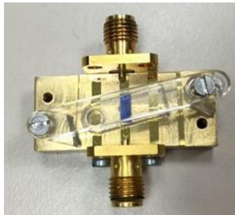
Figure 4.39 Photographic top view of a fabricated superstrate microstrip gapline switch
