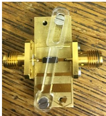
Figure 4.30 Photograph of a superstrate microstrip gapline with superstrate fixed by Perspex
