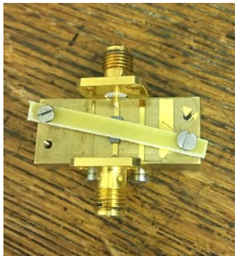
Figure 4.27 Photograph of a superstrate microstrip gapline with superstrate fixed by Duroid
