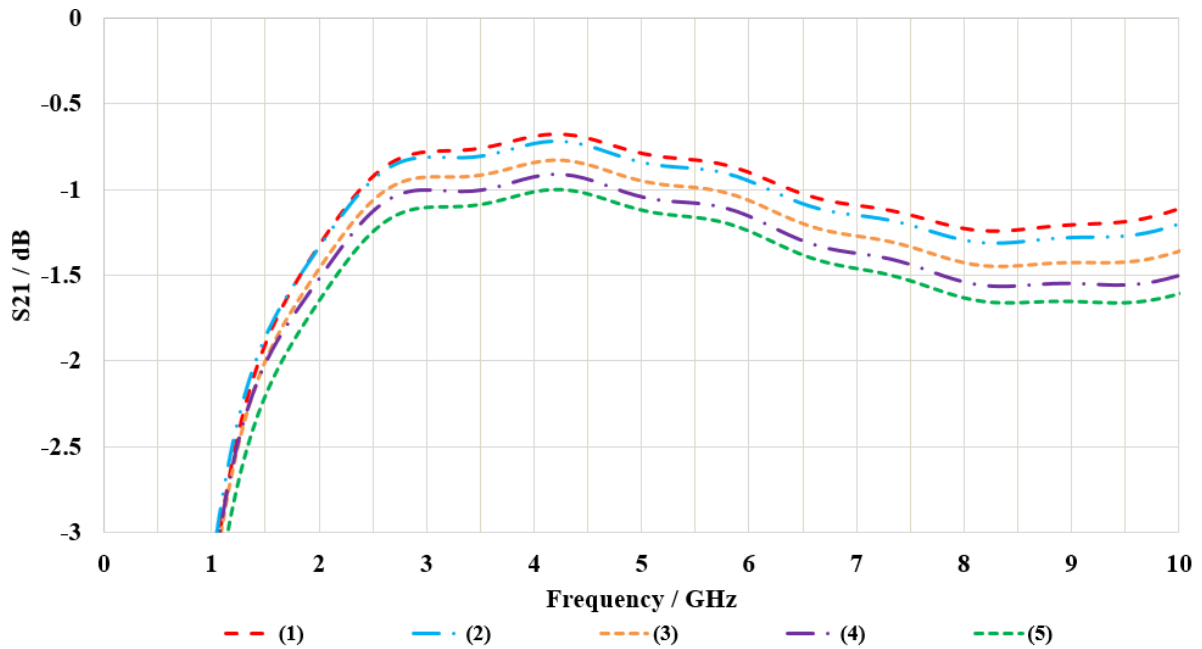
Figure 4.12 Simulated S21 results for a superstrate gapline of 1mm linewidth with varying gap lengths (1)0.1mm (2)0.2mm (3)0.3mm (4)0.4mm (5)0.5mm and surface plasma layer conductivity 1000S/m
