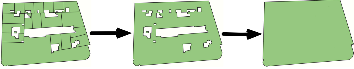
Figure 7.1: Example of how adjacent buildings (left), are concatenated to a single polygon (centre) at first, and the inside holes are removed (right), using the union polygon operation [4]. By that, we can decrease the execution time of our simulation.
