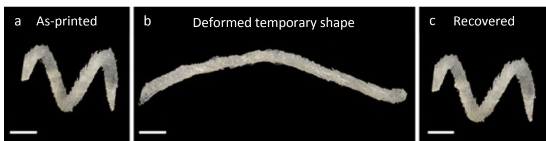
Figure 1.9: Actuation response of FFF printed spring demonstrating shape memory effect. (a) The spring as printed. (b) After the programming step of deforming at elevated temperature followed by cooling. (c) Recovered shape after heating by immersion in hot water at at 70 °C. (Scale bar = 10 mm). Image adapted from [103] with permission from ACS Publications.
