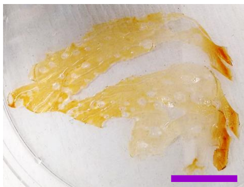
Figure 4.5: Cracking observed in PAA crosslinked samples after swelling. (Scale bar = 20 mm).
