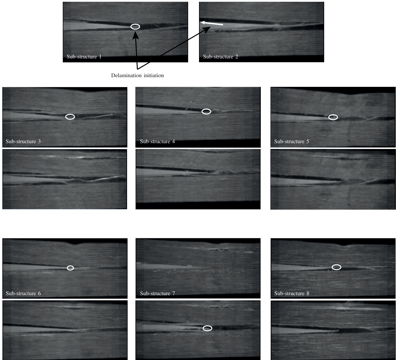
Fig. 11 High speed camera results. The upper image for all sub-structures shows the damage state after insert delamination except for sub-structure 7, and the lower image shows the damage state after wrinkle delamination except for sub-structure 1, 2, and, 7. The white circles indicate the delamination initiation point, the white arrow in sub-structure 2 indicates that initiation was outside the frame.
