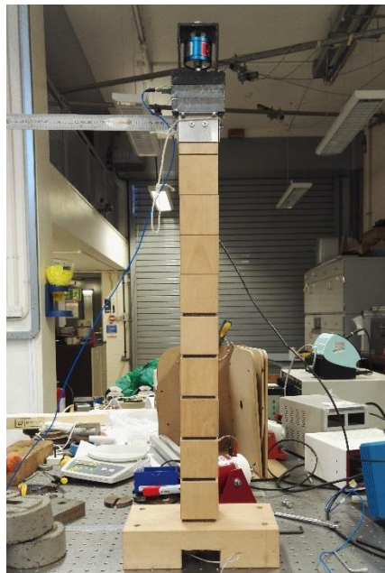
Figure 2. (a) Image of an entangled metal wire (EVM) sample used in the composite intervertebral disk, and (b) Example of small-scale self-centring vertebral columns with six intervertebral discs.
