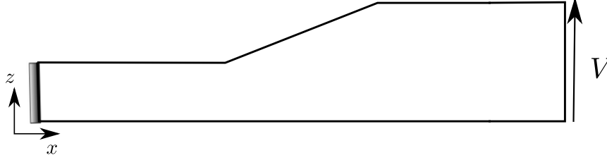
Fig. 4 Loading state utilised to obtain neutral plane's position using the UF-SLE model.
