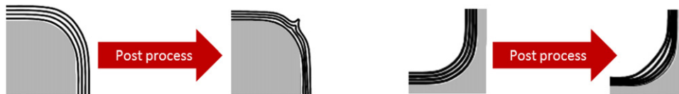
Figure 1. Left: convex corner defects (wrinkles), right: concave corner defects (bridging), adapted from [37].
