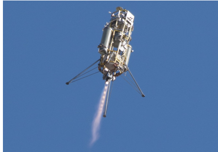
Figure 7: Photo of NASA's reusable VTVL platform Xombie demonstrating Mars-like descent and pinpoint landing [Credits: NASA/Tom Tschida]
