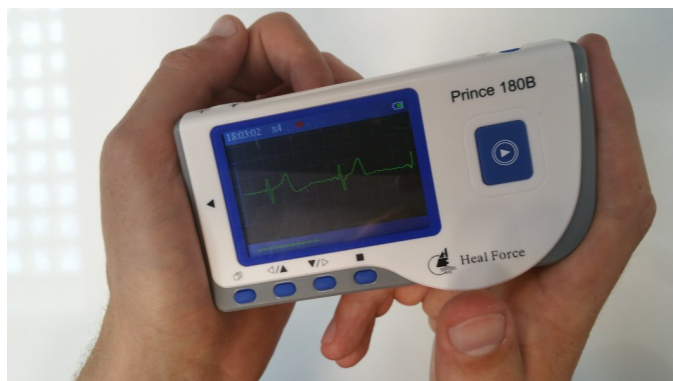
Fig. 8: ECG monitor in palm measurement mode
