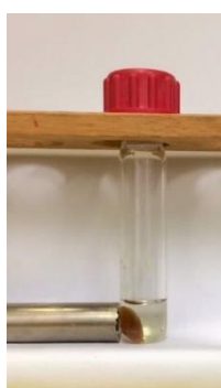
Figure 4.7. AFPMIL contacted with feed solution (0.1 M \text{HNO}_3 containing 250 ppm U (VI)), with the application of an external magnetic field.
