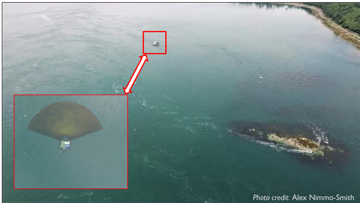
Figure 3. Minesto's site in The Narrows tidal channel with a M3 multibeam sonar swath set to 50m range mounted from Minesto's barge (insert), for scale visualisation of the hydroacoustic monitoring approach.
