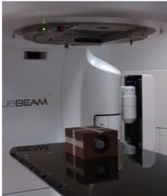
Figure 5.1: Phantom used for homogeneity experiments. 2.5cm WEP blocks were added on top and beneath the phantom.
