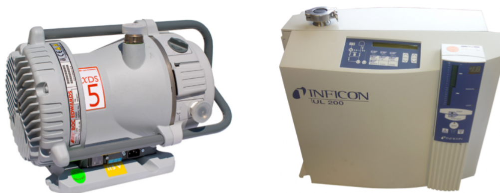
Figure 2.5: XDS5 scroll vacuum pump on the left [96] and Helium Leak Detector Leybold INFICON UL 200 [97].
