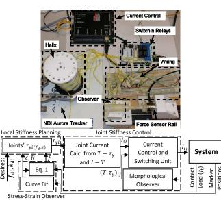
Fig. 4. (top) Experimental control setup, (bottom) a minimal central controller for model-based decentralized impedance regulation. The joint current calculation unit is replaced with a switching term in the case of a simple switching controller.
