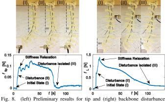
rejection through passive shape adaptation with three independent stiffness controllable elements: initial state (I), disturbance (II), effect isolation (III).
