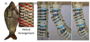
Fig. 1. (a) Overlapping and helical arrangement of scales in a Cyprinus Carpio fish, (b) the thermoactive interface integrated on a two module STIFF-FLOP continuum manipulator for stiffness control (left & middle) and shape locking (left & right) in the straight and bent configurations.
