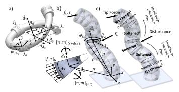
Fig. 3. (a) Free body diagram and kinematics of a full turn segment, (b) VC kinematics and Cosserat rod method parameters for a continuum manipulator, (c) sample information flow in a disentralized stiffness regulation strategy for impedance disturbance isolation in the <sup>1</sup>contacting element, <sup>2</sup>adjacent elements and <sup>3</sup>rest of elements.
