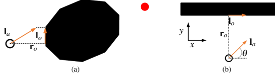
Fig. 2. (a) The workspace of a point-like robot moves towards the goal (red circle) in the vicinity of the polygonal obstacle (black). \mathbf{l}_o and \mathbf{l}_a denote the artificial current on the obstacle surface and the robot's velocity. (b) The scenario of a robot moving in the vicinity of a flat obstacle surface.
