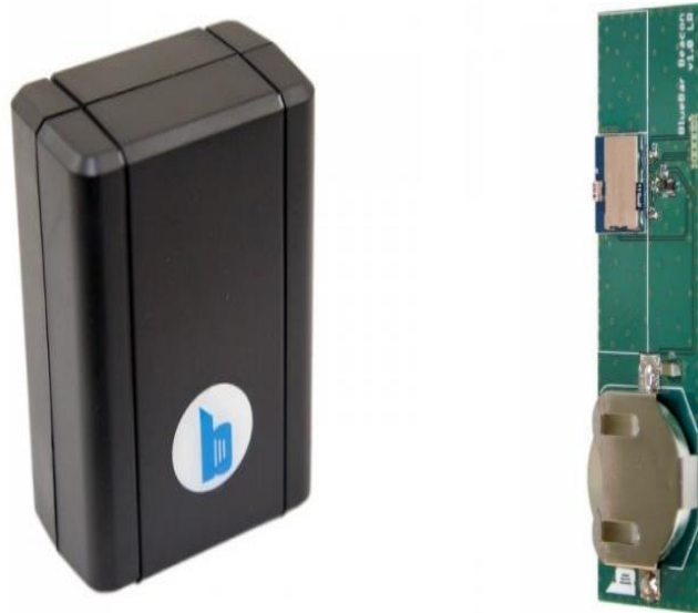
Figure 3-1 The Bluebar iBeacon device (7.5 cm * 5 cm)
