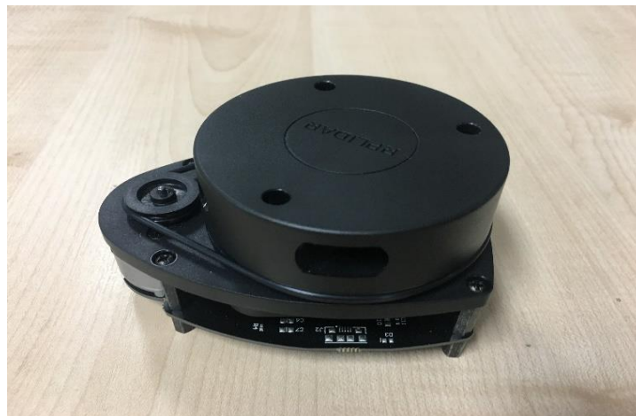
Figure 6-10 2D (PRLIDAR) Lidar IPS device
