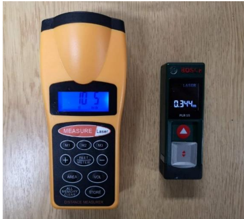
Figure 3-8 Laser tapes are used to determine the location ground truth
