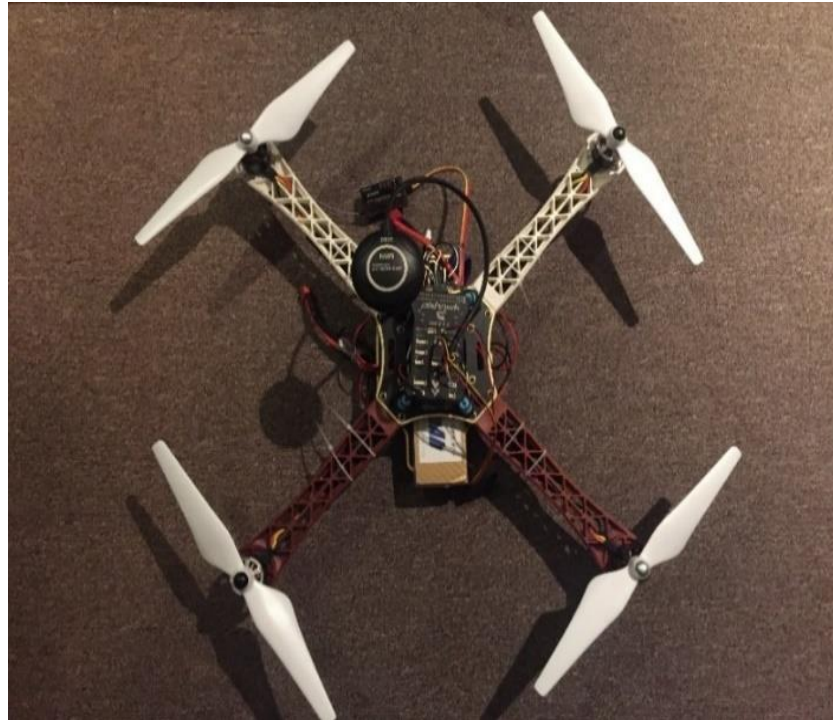
Figure 5-10 The office WiFi fingerprint collection drone (UAV)
