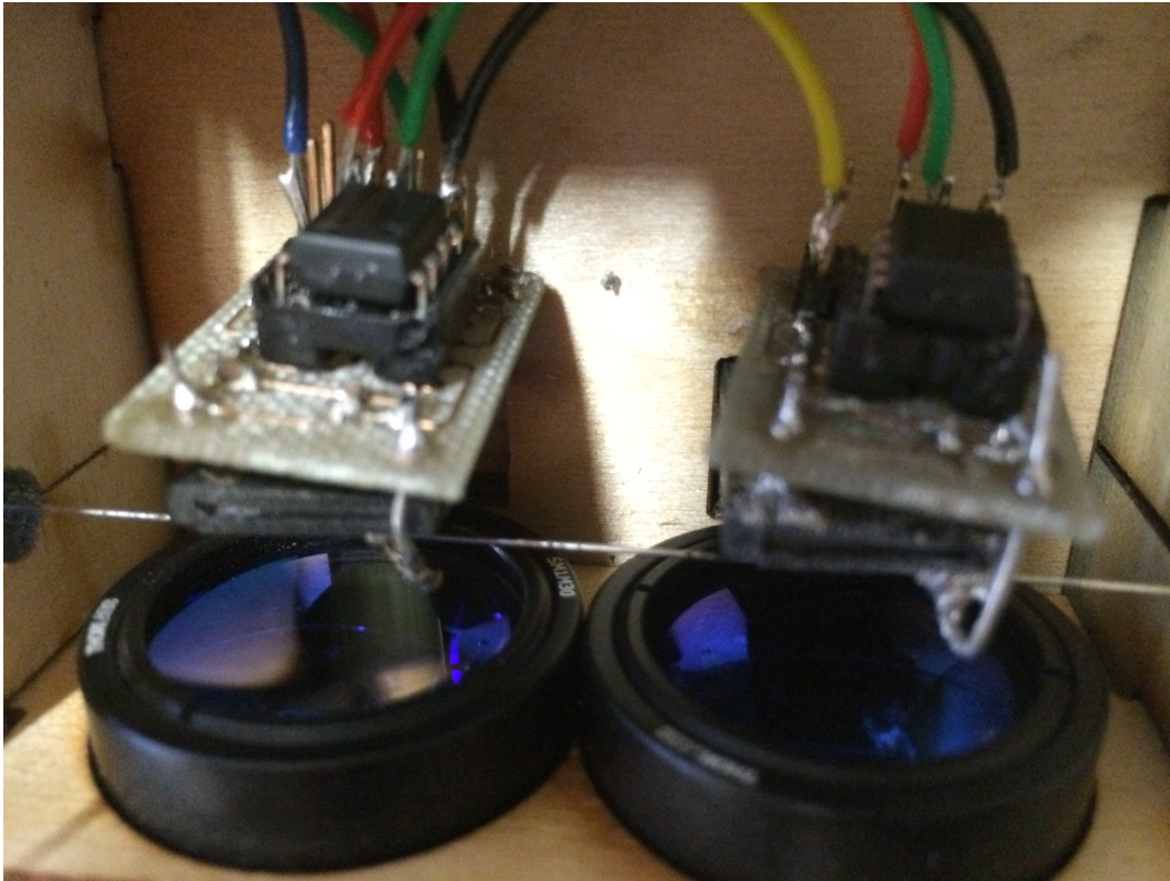
Figure C.5: Internal closeup of the sensor, showing the collimating lenses and the photodiode preamplifier circuits
