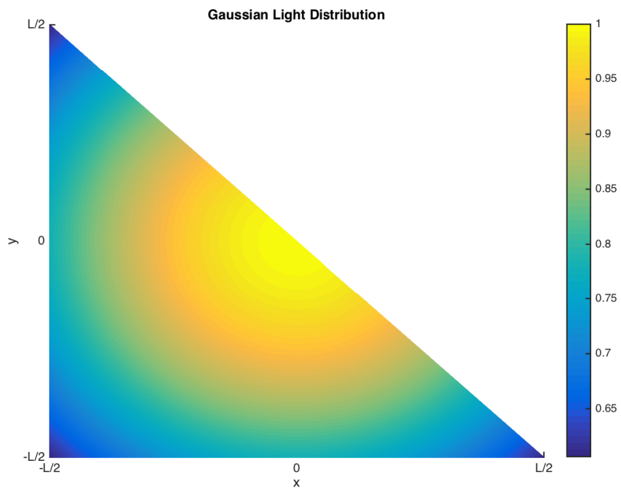
Figure 4.9: A two-dimensional gaussian light distribution with spread \sigma = \frac{\sqrt{2}}{2} projected onto a triangular sensor with dimension L = 1
