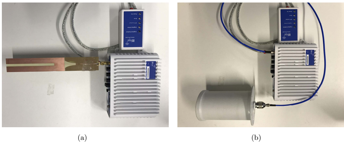
Figure 6.5: RFeye node with (a) the in-house developed antenna and (b) a commercial antenna.
