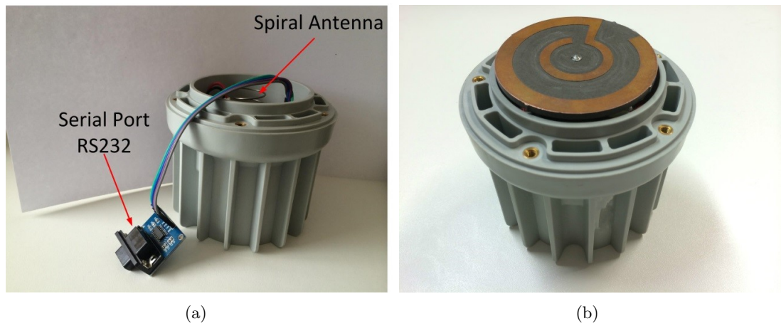
Figure 6.1: Sensor node with (a) a commercial spiral antenna and a serial port extension and (b) the in-house developed antenna.
