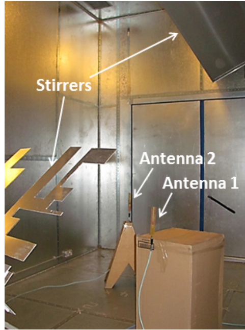
Figure 4.14: Set up of the antenna radiation efficiency measurement using two-antenna method in a reverberation chamber.
