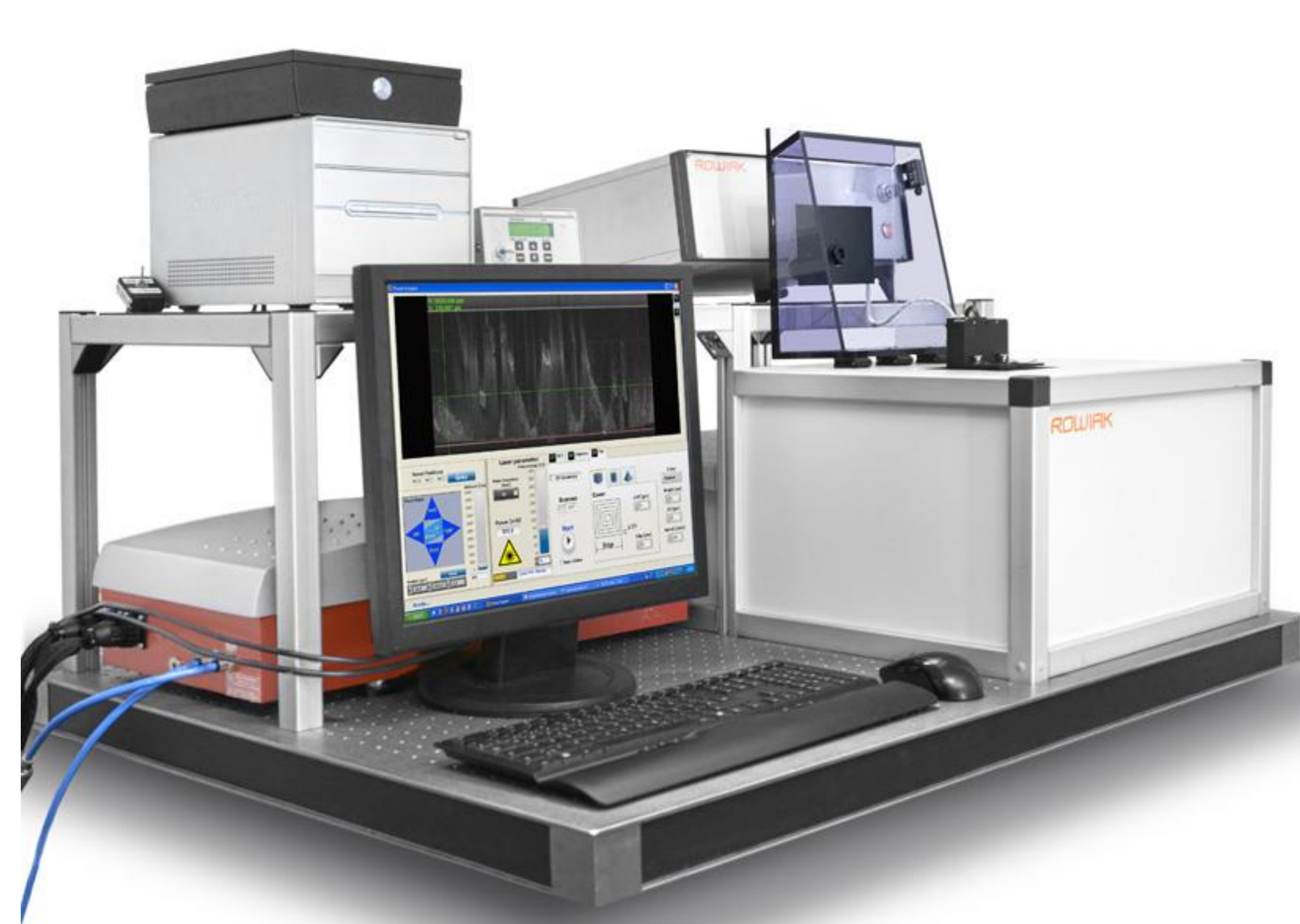
Rowiak LaserLabSolutions GmbH 'TissueSurgeon' laser microtome
