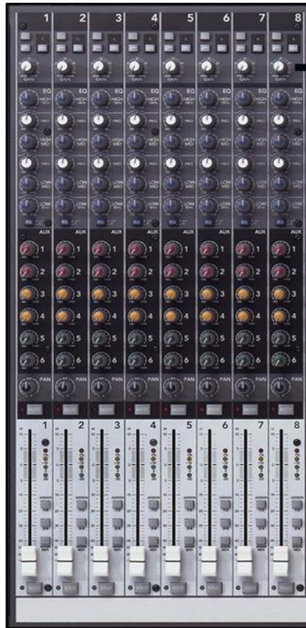
Figure 1:1: Mixing desk channel strips. Each channel typically contains controls for (top to bottom), microphone input level, equalisation, effects (auxiliaries), panning position and volume level. Common desk sizes include 8, 16, 24 and 32 channels.
