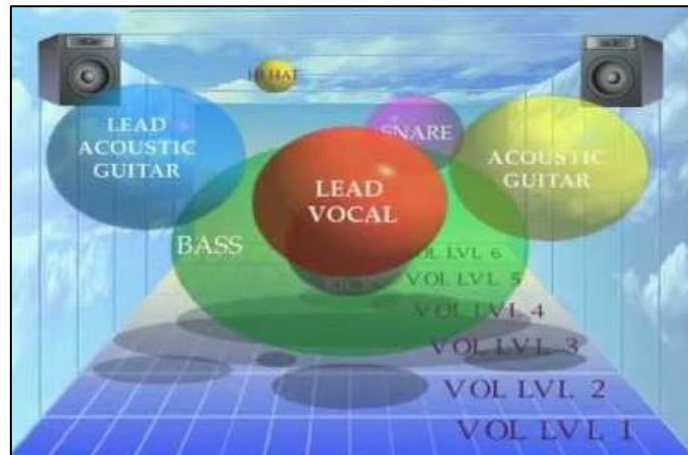
Figure 2:10: Though never realised as a working mixer, Dave Gibson uses the concept of the Stage Metaphor to analyse mixes and visualise ways of placing elements within a multi-channel mix. From Gibson (1997)
