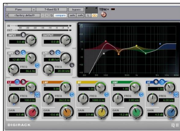
Figure 4:2: Pro Tools equaliser, version 6.9 onwards. The GUI is more complex, with colour coded dials and numeric information in addition to a graphical representation of the frequency curve.
