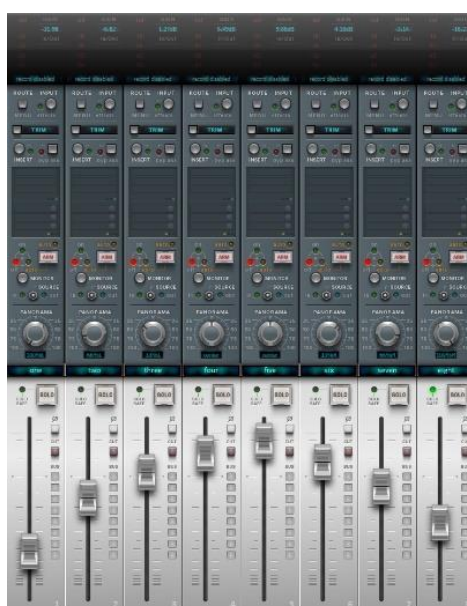
Figure 2:1: Reaper DAW mixer screen. Its design is closely modelled on an analogue mixing desk. However, unlike a physical desk, it offers potentially unlimited channels.
