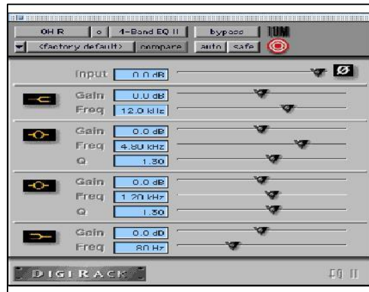
Figure 4:1: Pro Tools equaliser, version 5.1. Except for the sliders, there is limited visual feedback in the GUI design.
