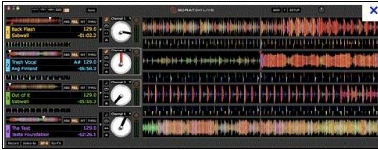
Figure 2:8: Serato uses coloured waveforms so that users can identify individual drum hits even at high zoom levels (darker colours are mapped to lower frequencies).
