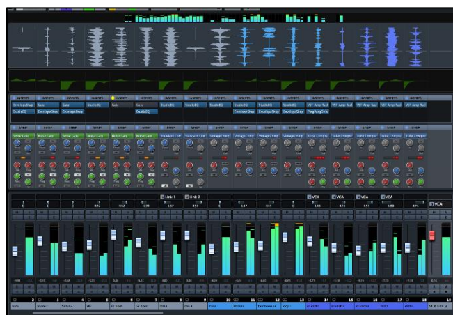
Figure 2:3: Cubase 9 mixer window. While still based on the CS metaphor, DAW mixers such as Cubase have extended the metaphor. For example, in Cubase 9, the mixer includes equalisation curves and waveform displays (at top of screen).
