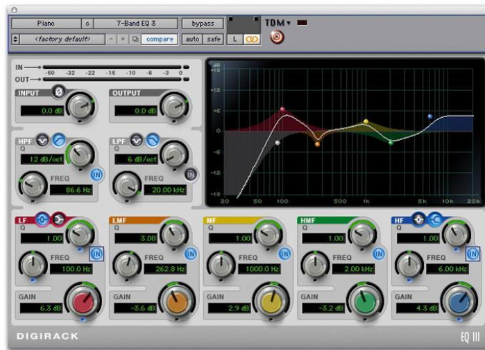
Figure 3:1: The Pro Tools channel EQ. The gain scale of +/- 18dB can potentially make small gain changes (in the region of 1 or 2 dB) seem visually insignificant. While some EQs allow rescaling of the gain axis (e.g. to show it as +/- 3dB) this is not possible here.
