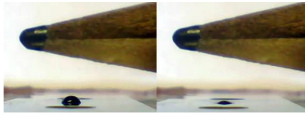
326 Fig. 9. Picture of a prototype Braille dot at rest (left) and when a voltage is applied (right). A video of the dot in action is available at
