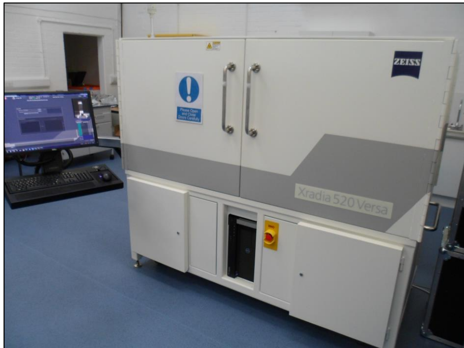
Figure 3-15: Photograph of the Zeiss Xradia 520 Versa 3D X-ray microscope at the Technology Centre of the University of Portsmouth, which has been used for the micro-CT scanning in this study.
