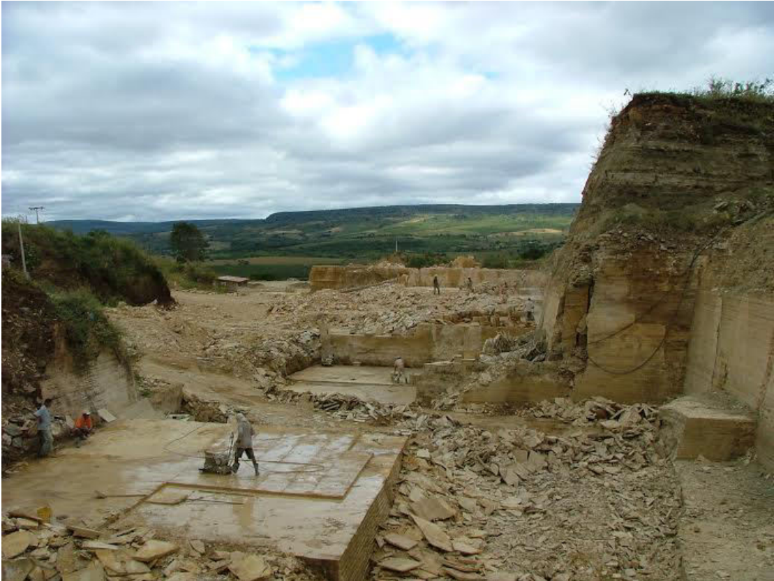
Figure 2. Photograph of the Crato Formation being quarried for paving slabs. Image © D. M. Martill, quarry location near Nova Olinda.
