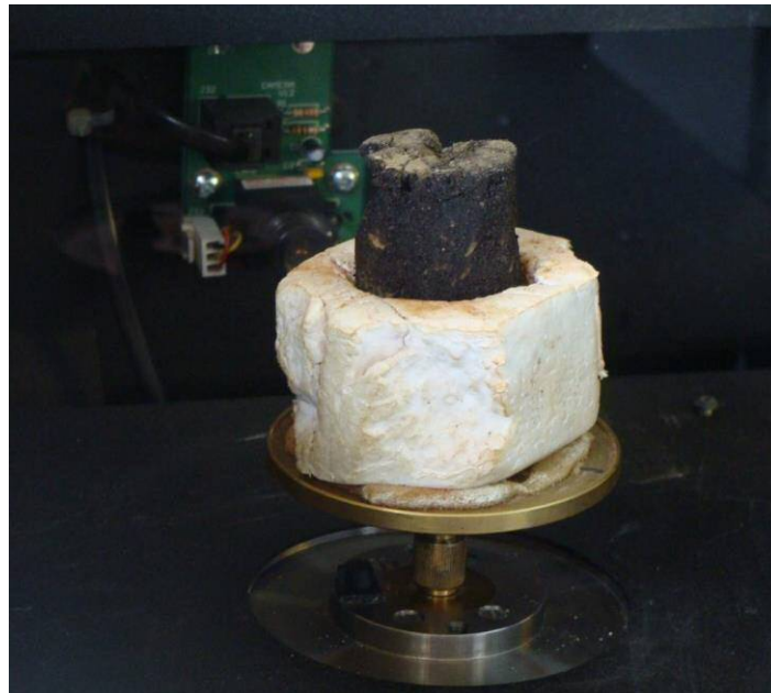
Figure 3-34 Part of the sample mounted on polystyrene holder and is ready to be scanned in micro -CT equipment.
