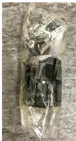
Figure 3-35 Part of sample held on stage and wrapped in Cellophane tape while scanning in Zeiss equipment.
