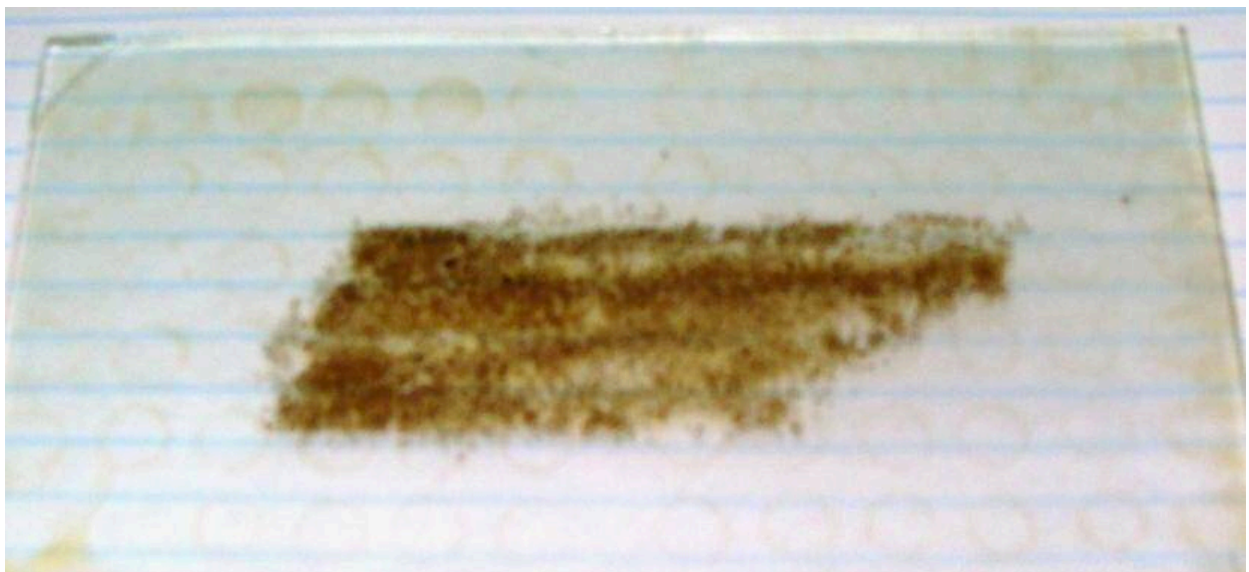
Figure 3-20 Sample grinded using water cooling
