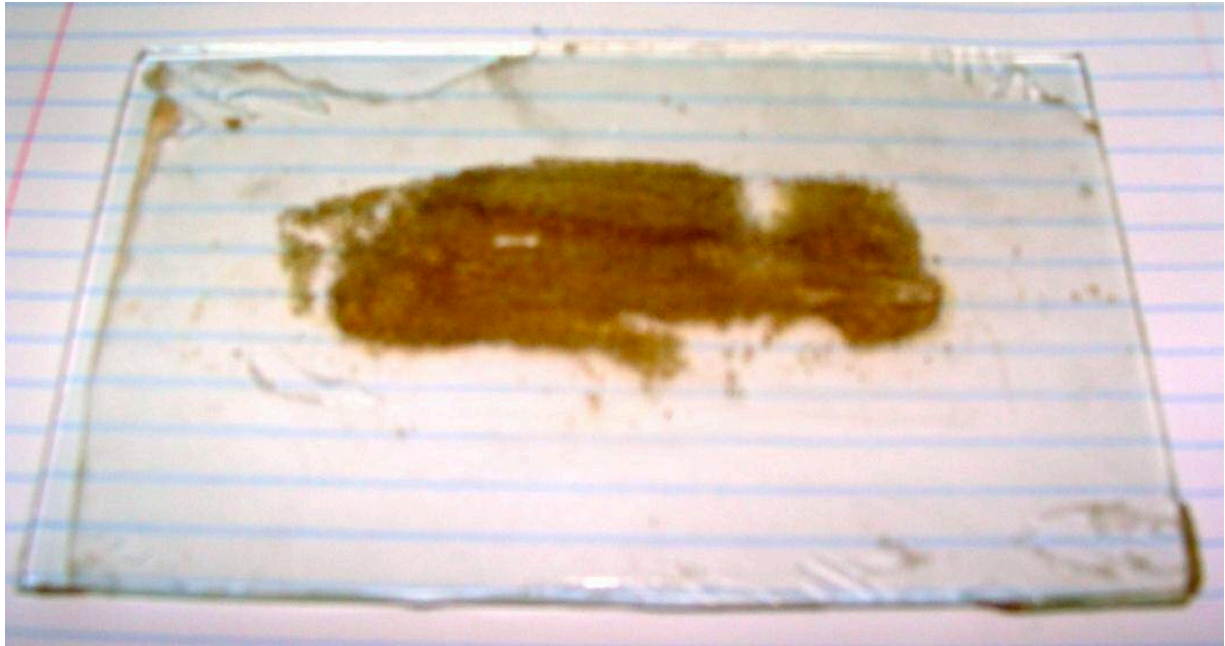
Figure 3-19 Sample grinded with ISOPAR cooling liquid
