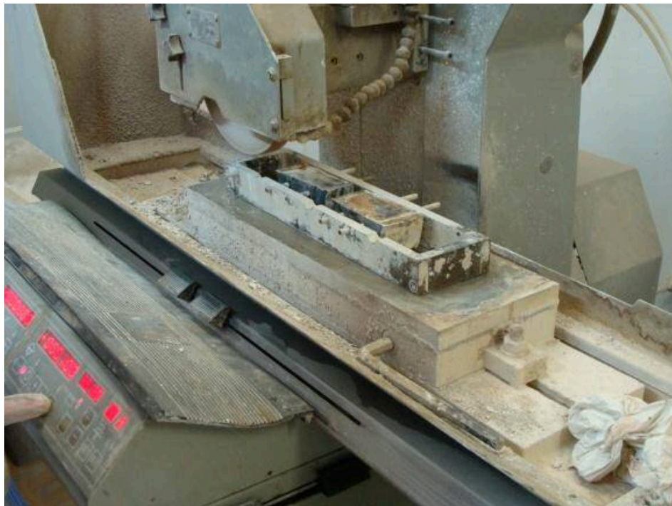
Figure 3-12 Surface grinder with rectangular support and sample
