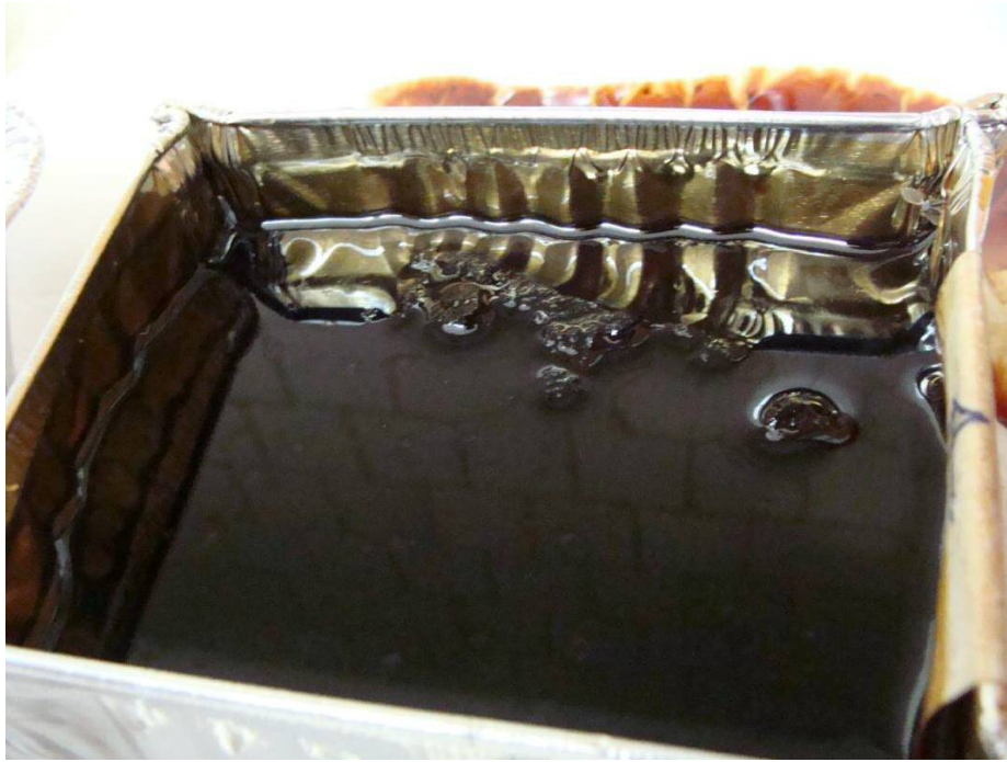
Figure 4-3 Sample undergoing Polymerisation using polyester resin.
