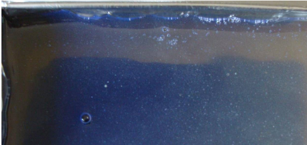
Figure 3-10 Vacuum process working as air bubbles can be seen leaving the resin dipped sample.
