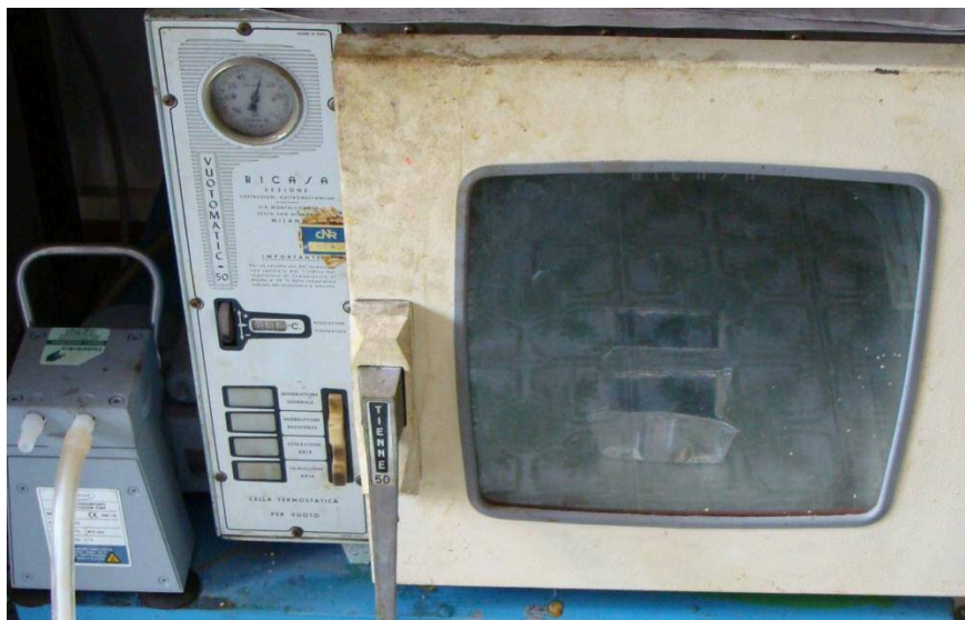
Figure 3-9 Vacuum chamber used for this experiment to reduce amount of air
