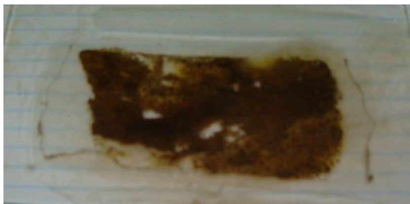
Figure 4-4 Thin section prepared using standard epoxy based polymer, re-impregnation and regrinding using water based coolant
