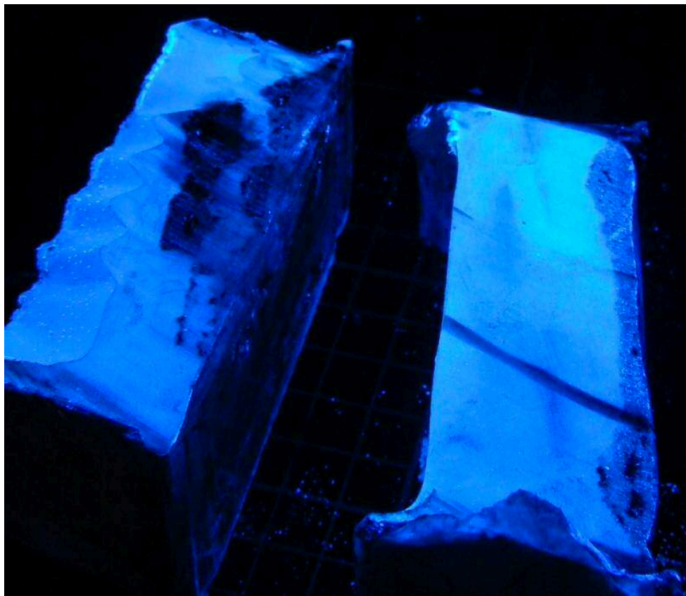
Figure 3-11 Sample being subjected to UV light to accelerate polymerisation process.
