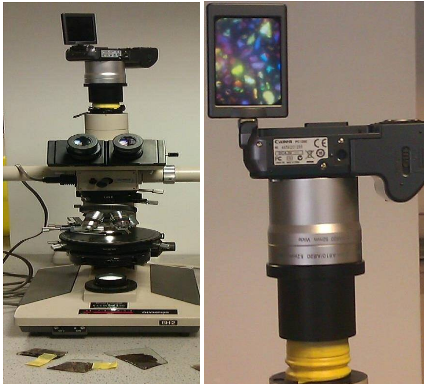
Figure 3-21 Microscope and camera setup with an attachment to capture thin section Images
