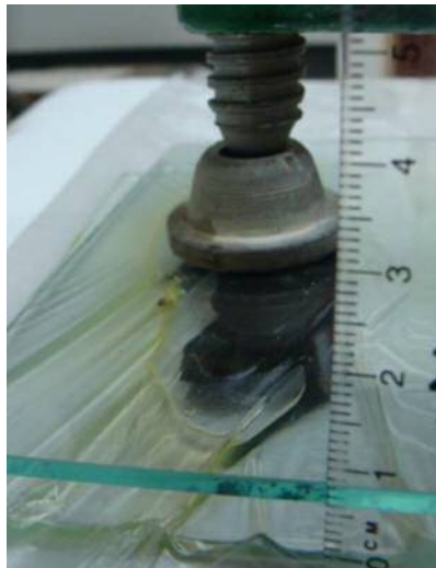
Figure 3-17 Sample being bonded to the glass piece for preparation of thin section
