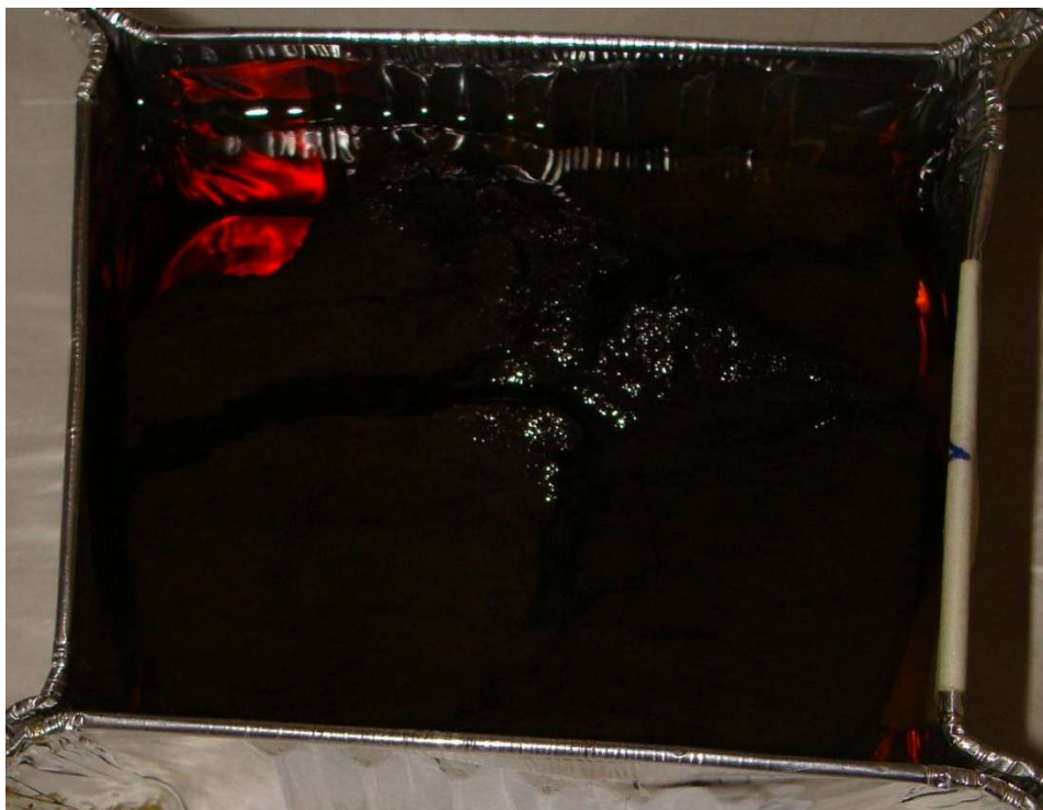
Figure 4-2 Sample losing bitumen when subjected to Acetone
