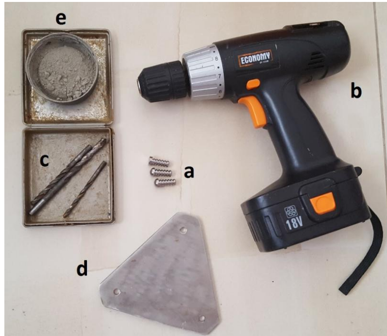
Figure 3.6: Tools for the installation of TMEM stations: a. Titanium studs; b. Cordless driller; c. Twist drill bits; d. TMEM position plate; e. cement powder (Source: Photo taken by Author)
