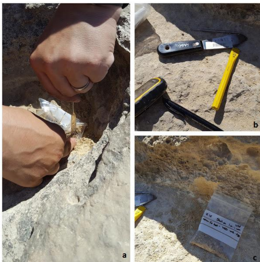
Figure 3.12: a. Extraction of sample from the platform surfaces ; b. Field tools used for the extraction: GPS, two geological chisels, and sample plastic bags; c. An example of a packed sample extracted from in situ close to MRF Station 1b, Ras il-Fenek (Source: Photos by Author)
