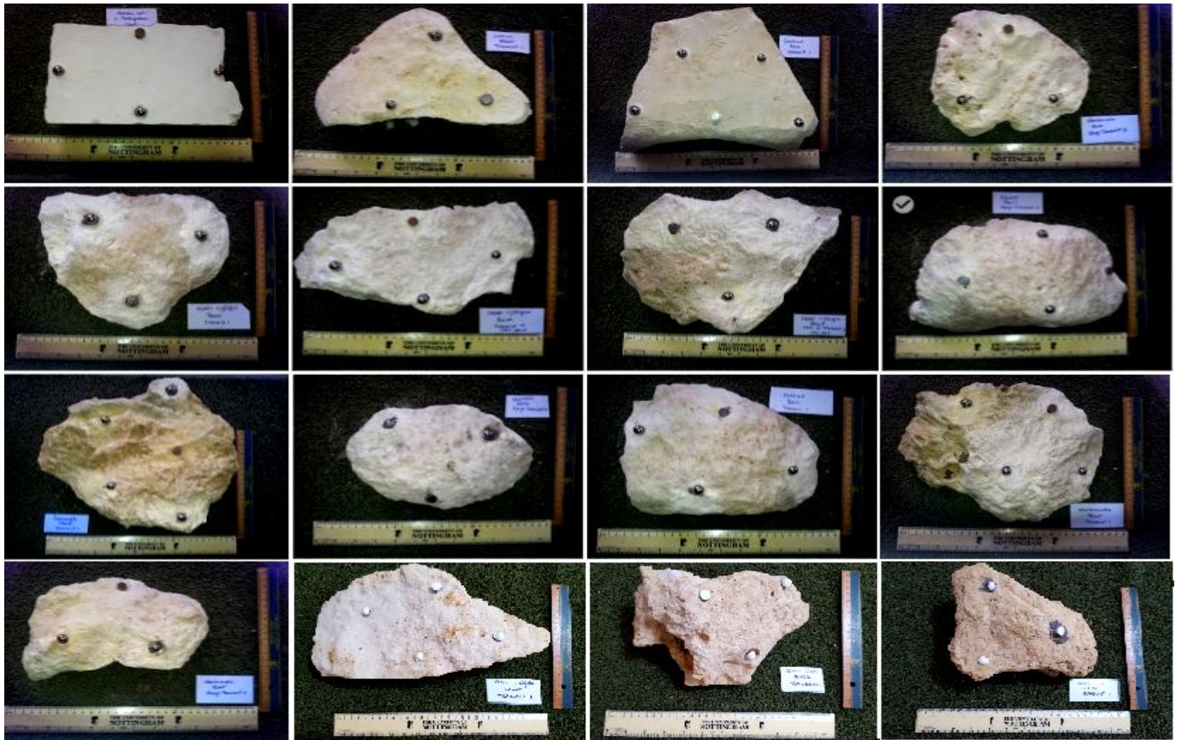
Figure 3.9: Sixteen experimental slabs prepared with TMEM stations to measure surface rock erosion by sub-aerial weathering (Source: Photos taken by Author)
