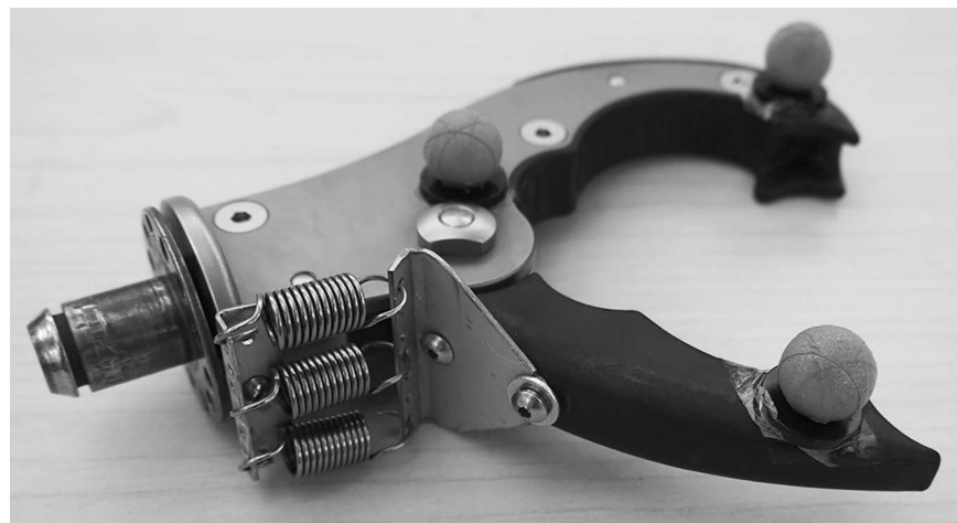
Fig 2. Prehensor. TRS hook with the internal torsion spring replaced by external linear springs in the high force setting (3 x 1.7 N/mm springs); 2 x 0.11 N/mm springs were used for the low force setting.
