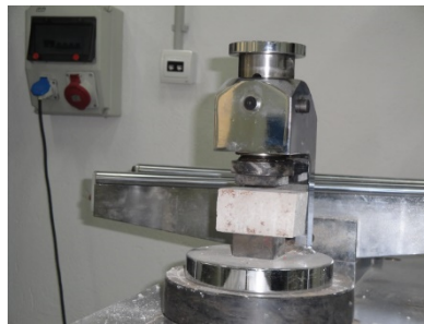
361 362 363 364 365 366 367 368 369 Figure 8. Charging device cubic specimens for compressive
