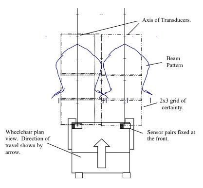
Fig. 3. Representation for a two-sensor array.
