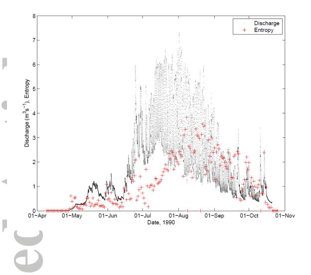
Figure 2. Daily entropy values superimposed on a discharge hydrograph for the Haut Glacier d'Arolla for the year 1990.
