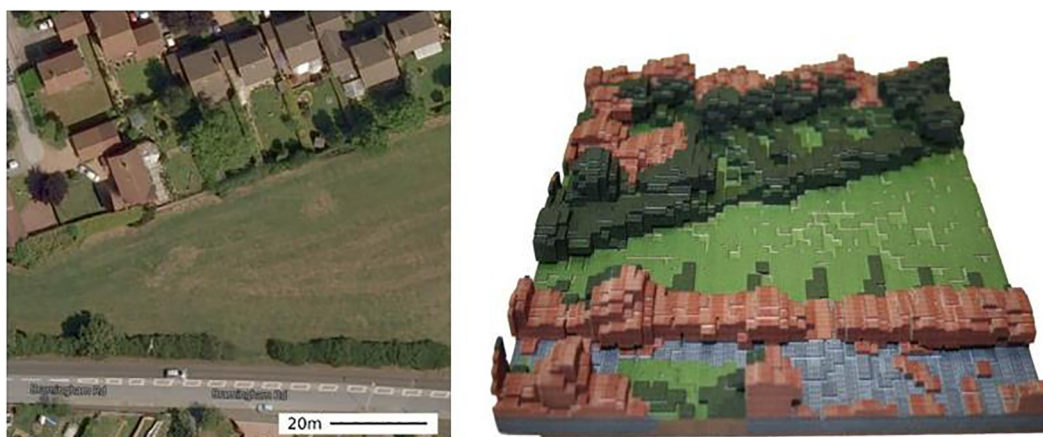
Fig. 8. Full colour sandstone 3D print, 170 × 180 mm, from Minecraft .obj file, Luton shown alongside an aerial photograph of the site. Colours are representative of the classifications in the voxel data – brown buildings, grey roads, pale green grass, mid-green shrubs and dark green trees. (For interpretation of the references to colour in this figure legend, the reader is referred to the web version of this article.)
