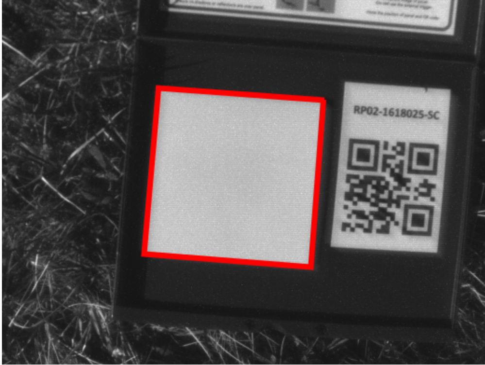
Figure 8: Parrot Sequoia pre-flight radiometric calibration image of a MicaSense Ltd. (Seattle, WA, USA) reflectance target in the near-infrared band. Red box: surface with known reflectance value used for calibration.
