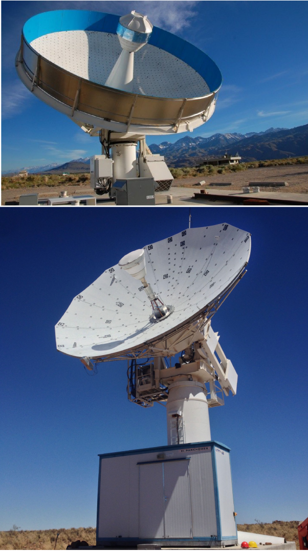
Figure 3. Top: The C-BASS North telescope, located at the OVRO in California, U.S.A. Bottom: The C-BASS South telescope, located in the Karoo desert, South Africa. The weather shield around the receiver is removed in this image, showing the lower part of the feed horn and cryostat.
