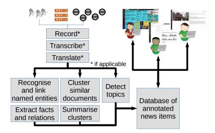
Figure 1: The SUMMA Platform Workflow
