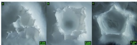
Fig. 18 Different 3D structures electrospun with the optimal parameters: 15.0 wt% PS in 1 : 1 DMF/THF electrospun at a voltage of +15-20 kV, a working distance of 5 cm, a flow rate of 5.0 mL h -1 and a nozzle speed of 12 mm s -1 for 10 minutes. (a) Triangle. (b) Square. (c) Five-pointed star polygon.
