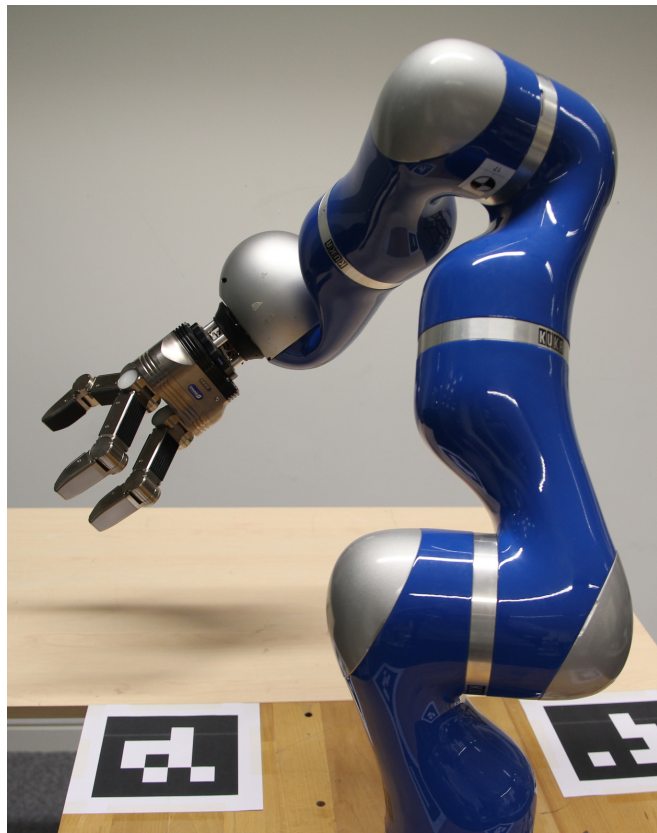
Fig. 5: KUKA LWR 4 (7DOF) with Schunk SDH2 (7DOF) mounted on a table with AprilTags for camera pose estimation.
