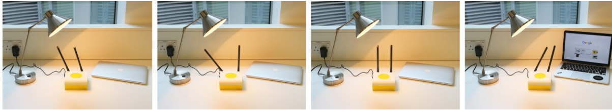
Figure 5 The gatekeeper monitors the data traffic within the machine network and indicates its working state by shaking its antennas.
