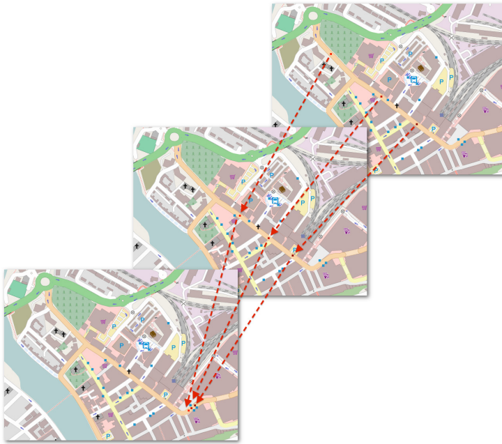
Fig. 9: Because of delays caused by boarding passengers the headway between buses is successively eroded over time until the buses are essentially working as a conglomerate.
