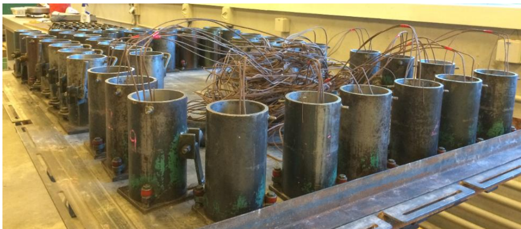
Figure 3. Photo of moulds for both series ready for casting on the vibrating table.
