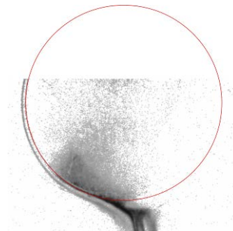
Figure 4: Light-sheet picture of the rhodamine concentration in the center plane of the sphere. A red circle indicates the contour of the sphere and next to it the boundary layer (thickness is about \delta/D = 0.023 ).
