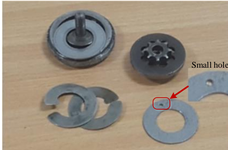
Figure 4-20 Leak in 2 nd stage discharge valve plate
