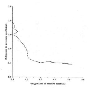
Figure 12: Difference between computed and experimental pressure coefficient against minus the logarithm of the relative residual.
