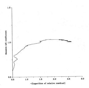
Figure 10: Relative lift coefficient against minus the logarithm of the relative residual.
