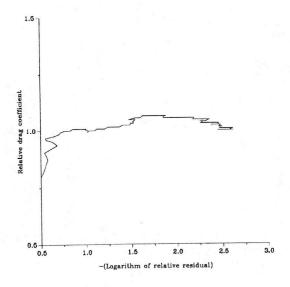
Figure 11: Relative drag coefficient against minus the logarithm of the relative residual.
