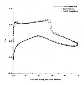
Figure 13: Various pressure coefficient profiles for the RAE2822 case.
