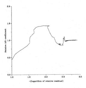
Figure 4: The relative lift coefficient against minus the logarithm of the relative residual.
