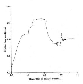
Figure 5: The relative drag coefficient against minus the logarithm of the relative residual.
