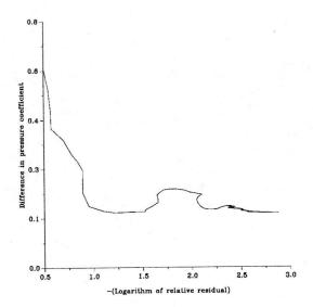
Figure 6: The norm of the difference between the computational and experimental pressure coefficients against minus the logarithm of the relative residual.
