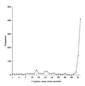
Figure 2: The frequency with which the largest residual occurs in a cell which has a particular j index. A cell in which j = 1 is next to the aerofoil (or the wake cut), whilst a cell in which j = 32 is next to the far-field boundary.
