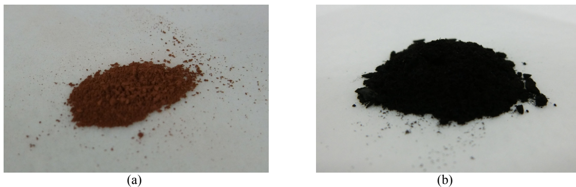
FIGURE 8. Photographs of (a) ash and (b) remaining powder after MeOH decantation in pyrolysis oil generated during 24 h operation.
