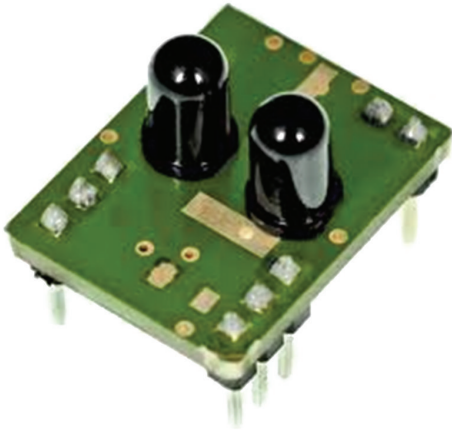
FIGURE 4: IR proximity sensor module.
