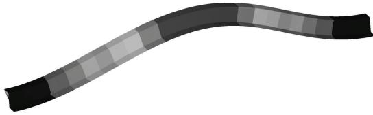
FIGURE 10: First buckling mode of half corrugation.
