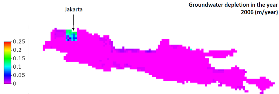
Figure 3. Screen shot of revised depletion ( \text{m yr}^{-1} ) results as calculated by the global hydrology model for the island of Java, Indonesia. It shows the depletion of the groundwater as a result of ground water abstraction in the urban area of Jakarta. The calculated depletion in the irrigation areas is now minor.
