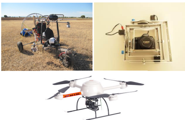
Figure 1. Paratrike employed (up-left); detail of the stabilization platform "MUSAS" (up-right) and UAV used in those complex areas (down).
