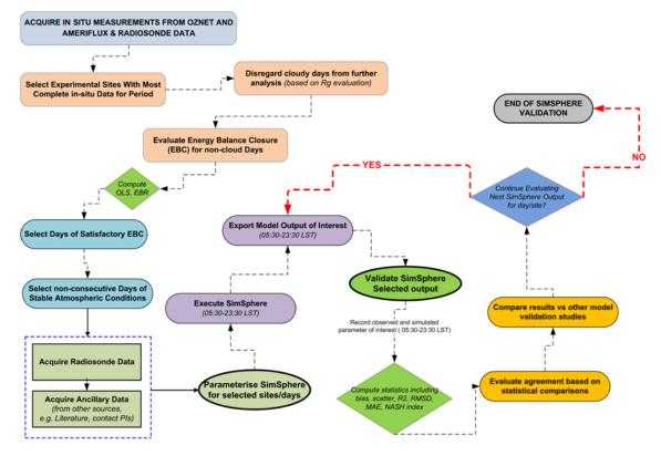
Figure 1. Flowchart of the overall methodology followed in evaluating SimSphere's outputs.
