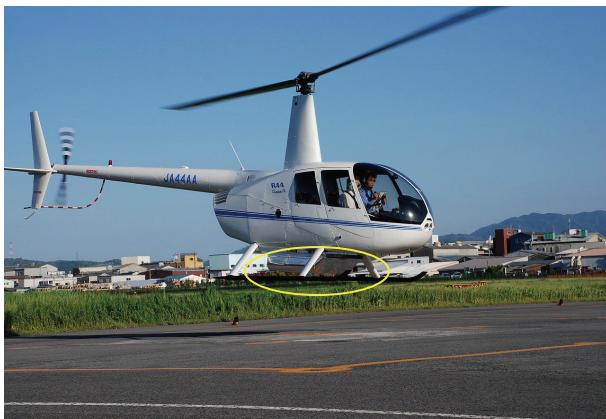
Fig 2. Helicopter(R44) and Laser scanner system
