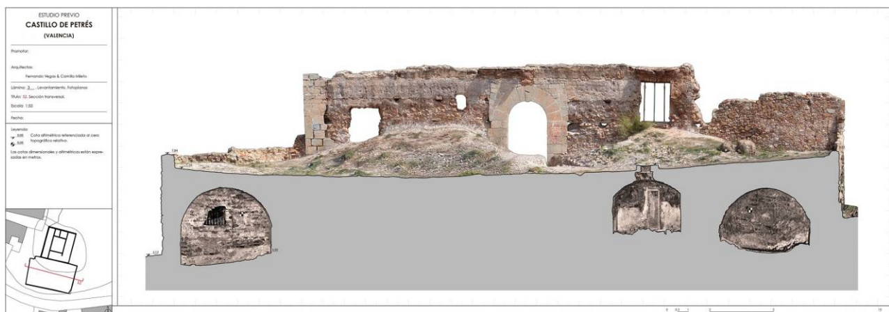
Fig. 6. Drone + scanner-laser: Section of the Castle of Petrés (Valencia, Spain)
