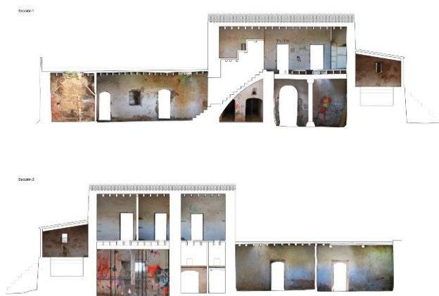
Fig. 3. Semi-manual survey. Sections of Can Ramón (Formentera, Spain)
